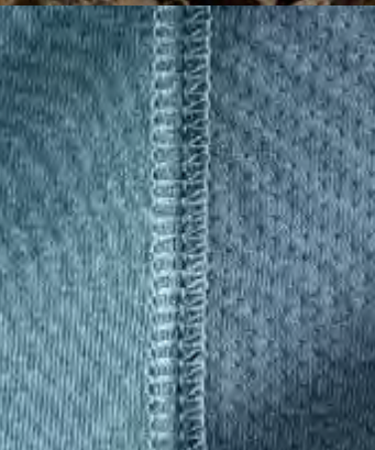
FLATLOCK SEAMS provide strength, minimize bulk, and reduce chafing for maximum comfort
